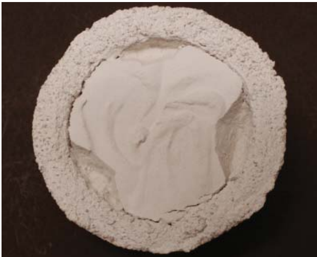
Fig. 3b: Shrinkage test. Plaster cup filled with grout: the grout has been excavated to assess shrinkage in depth; it shows shrinkage at the surface (probably related to fast evaporation), but not in depth (Pasian 2017©)
