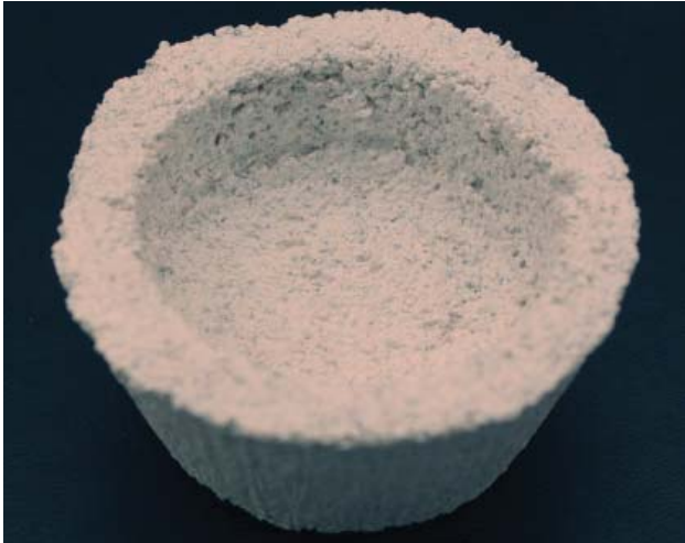
Fig. 3a: Shrinkage test. Plaster cup simulating a plaster pocket (Pasian 2017©)
