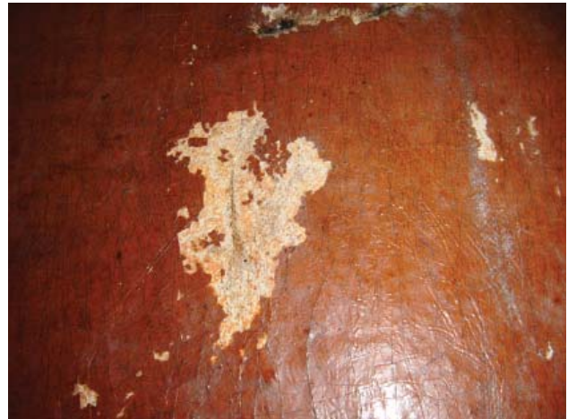
Fig. 15: Surface damage – loss of paint layer from being rolled during working life
