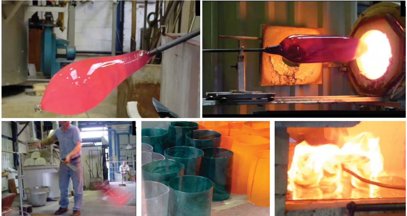
Fig. 7: Cylinder glass process
